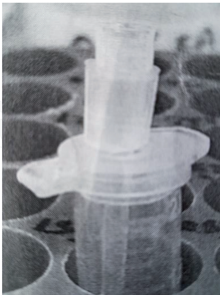
Figure 3. Shows a 2 ml pipette-tip (STAGE tip) inserted through a hole drilled into the top of a 2 ml collection tube. The pipette tip with SDB-RPS disk was inserted into the Eppendorf tube through the hole. Cell solution was pipetted from the top into tip so peptides could react with the SDB-RPS disk for 10 minutes.
